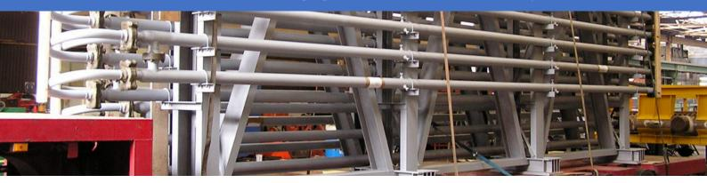
The Low-Density Polyethylene (LDPE) industry plays a crucial role in manufacturing a wide range of products, from plastic bags to packaging materials. One of the pivotal elements in ensuring efficient and safe LDPE production is the use of jacketed high-pressure (HP) pipework. This specialized piping system is designed to handle extreme pressures and temperatures, making it indispensable in the LDPE manufacturing process.
