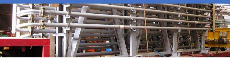
Unit Superheater Engineering Ltd is a leading manufacturer of jacketed HP pipework for the LDPE industry worldwide. Their expertise and innovative approach set them apart in the market, as evidenced by their recent fabrications adhering to the ASME B31.3: 2020 Design Code. By utilizing advanced materials like Nickel-Chrome for the inner tubes and Carbon Steel for the outer jackets, they ensure exceptional durability and performance.
