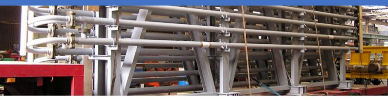
Unit Superheater Engineering Ltd, a part of UnitBirwelco, is a leader in manufacturing jacketed high-pressure pipework for the LDPE industry.
